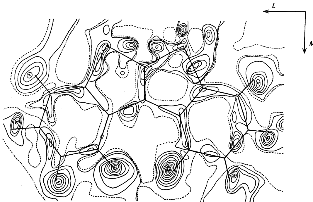
Fig. 3. Best plane section through the three-dimensional difference density. Contours at intervals of 0.05 e.Å -3 . Zero contour is represented by a dashed line. Heavy lines denote the projection of the molecule on the best plane after the completion of refinement.
